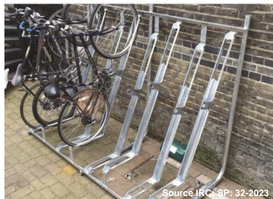
Figure 20 Racks for stacking and parking bicycles
