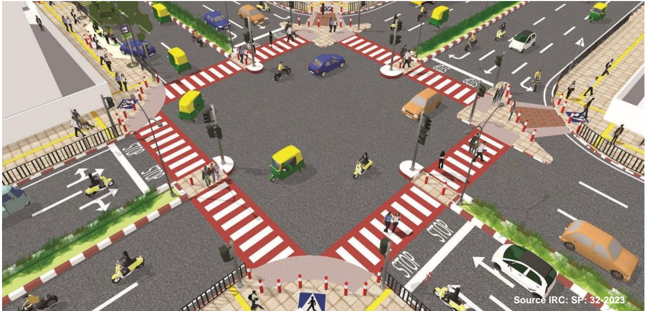
Figure 16 Intersection falling within a school zone
