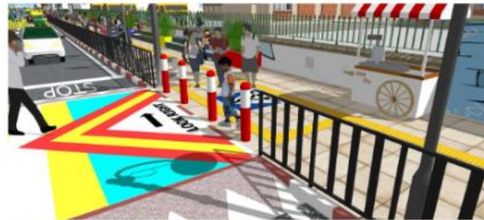
Figure 5-13: Guard rails and organisation of pedestrian space (projected cycle wheels are potential accidental hazard to children/ adults with visual impairment. Walkway shall show tactile paver 600mm away from the cycle wheel)
