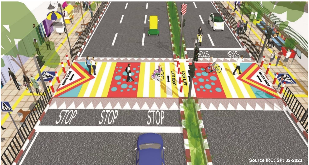
Figure 17 Speed table crossing
